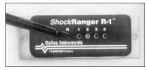
**Photo 1.** Dallas Instruments' R-1 ShockRanger, containing a piezoelectric sensor and powered by a lithium/thionyl chloride wafer cell, records maximum shock experienced by shipment of delicate goods.
