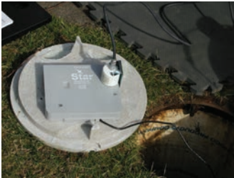
AMR/AMI meter transmitter units (MTU) are often buried underground, exposed to extreme temperatures and difficult to access for replacement.
