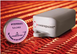
*Bobbin-type LiSOCl<sub>2</sub> batteries allow medical RFID tags to undergo high temperature autoclave sterilization without having to remove the battery.*
