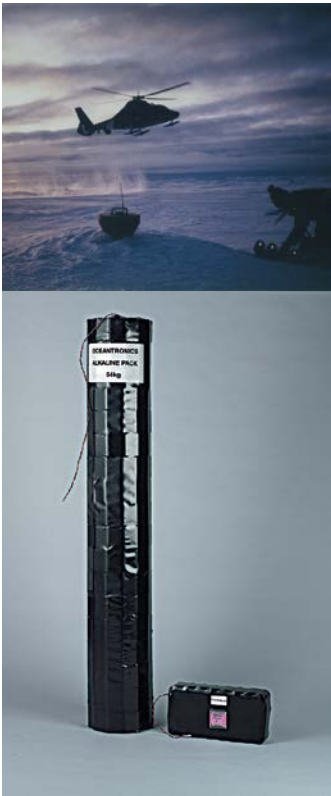
Converting to PulsesPlus battery packs reduced the size of a device that monitors the size and location of icebergs. The larger battery pack (left) used 380 D-size alkaline cells while the far more compact battery pack (right) used 32 lithium D-cells and 4 AA-sized hybrid layer capacitors (HLCs).
